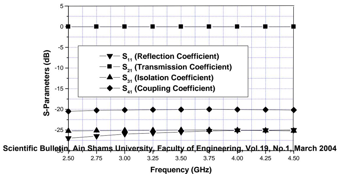
Fig.3 The simulated S-parameters for the microstrip three-section coupler
