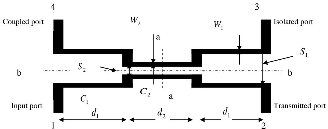
Fig.2 The three-section microstrip coupler
