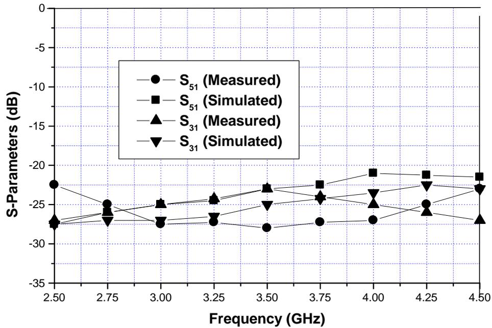
Fig.6 The measured and simulated  $S_{51}$  and  $S_{31}$  for the realized six-port reflectometer
