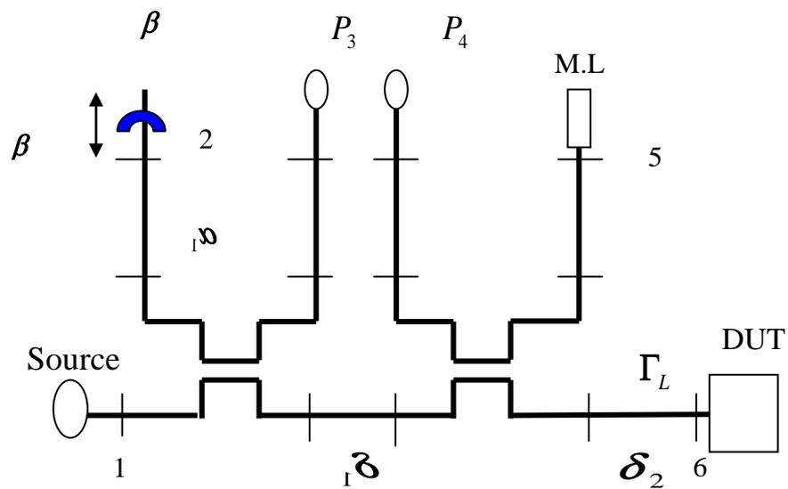
Fig.4 Six-port reflectometer using two microstrip three-section couplers
