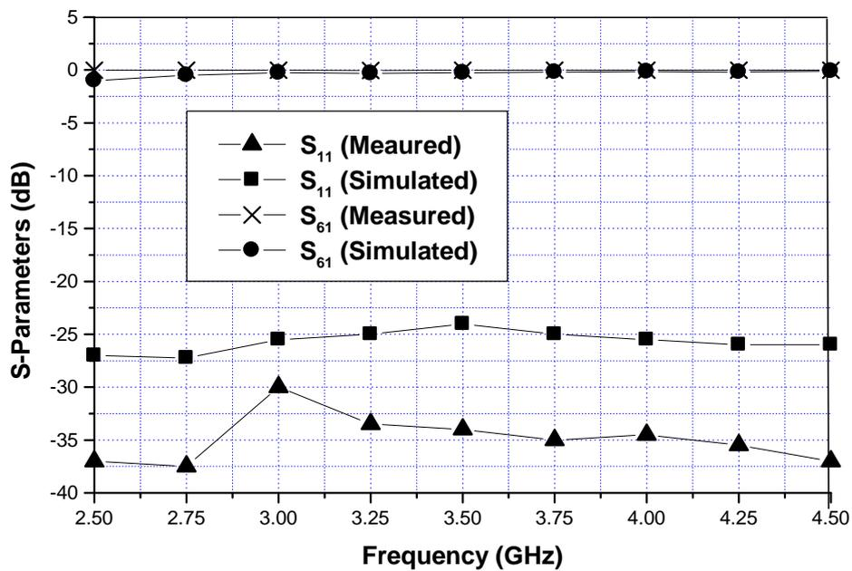
Fig.5 The measured and simulated  $S_{11}$  and  $S_{61}$  for the realized six-port reflectometer
