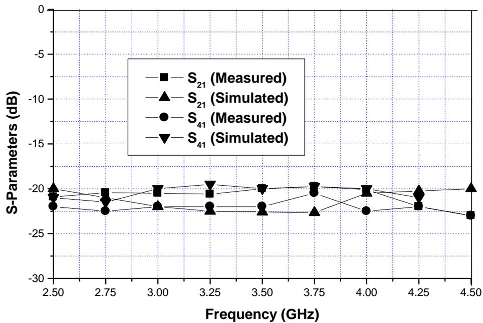
Fig.7 The measured and simulated  $S_{21}$  and  $S_{41}$  for the realized six-port reflectometer
