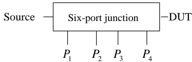
Fig.1 Six-port reflectometer
